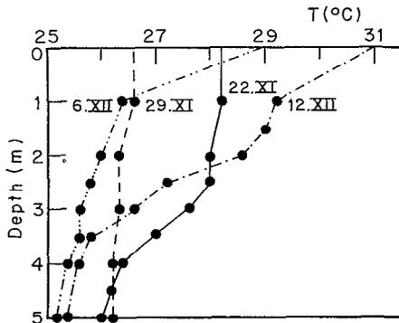
FIG. 7. — The arrival of a Polar Front on 22.XI.85, and the influence of its disturbances on the reservoir thermal stratification.
