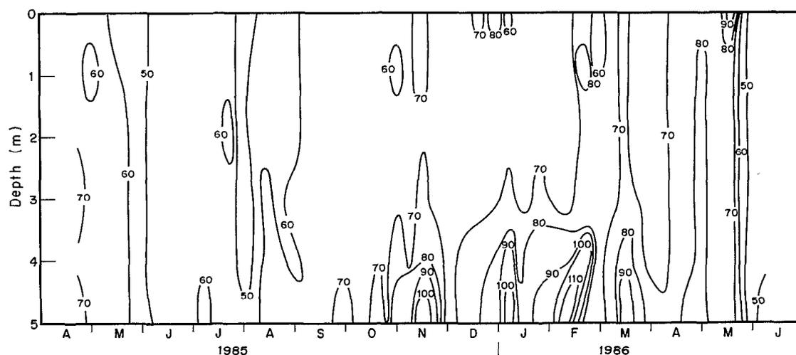
FIG. 9. — Depth-time diagram of conductivity isopleths, at intervals of  $10 \mu\text{S}\cdot\text{cm}^{-1}$ , from April 1985 to June 1986.
