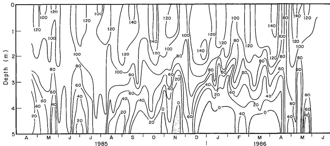
FIG. 5. — Depth-time diagram of dissolved oxygen isopleths, in per cent saturation, from April 1985 to June 1986.
