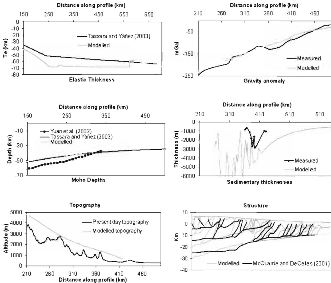
Figure 2: Comparison of our model results and elastic thickness, gravity anomaly, Moho depths, sedimentary thicknesses, topography and structure for the final stage (0 Ma) for elastic-plastic rheology.
