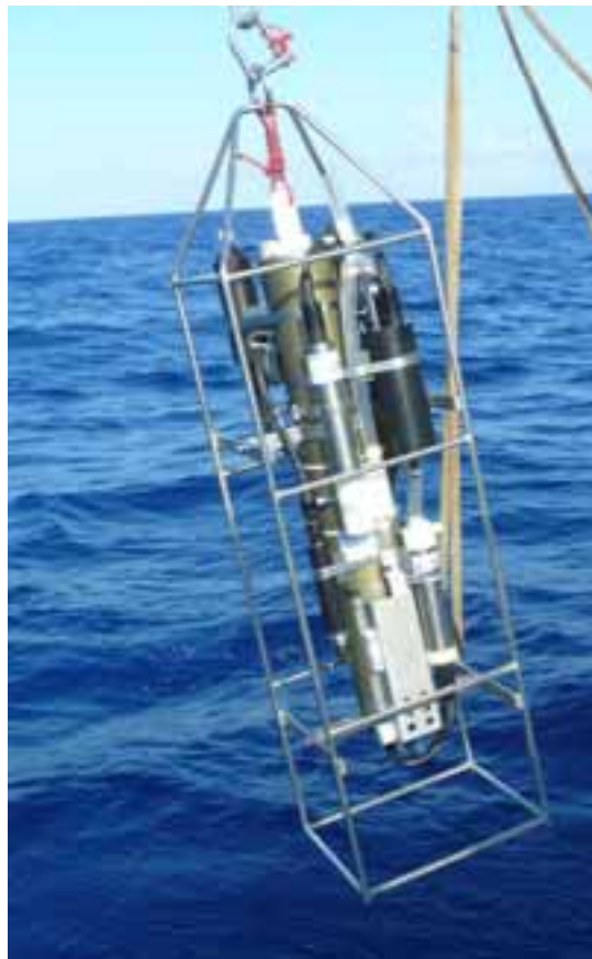
Figure 2 – Deployment of the CTD probe SEABIRD Seacat SBE19plus
