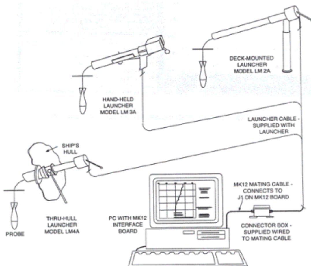
Figure 3 – Design of the Sippican's XBT system used to carry out temperature – depth profiles (Source : <http://www.sippican.com>).
