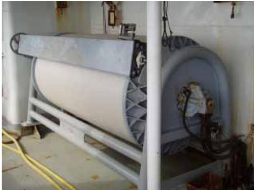
Figure 5 - The mainline spool by Lindgren Pitman™ installed on board the longliner
