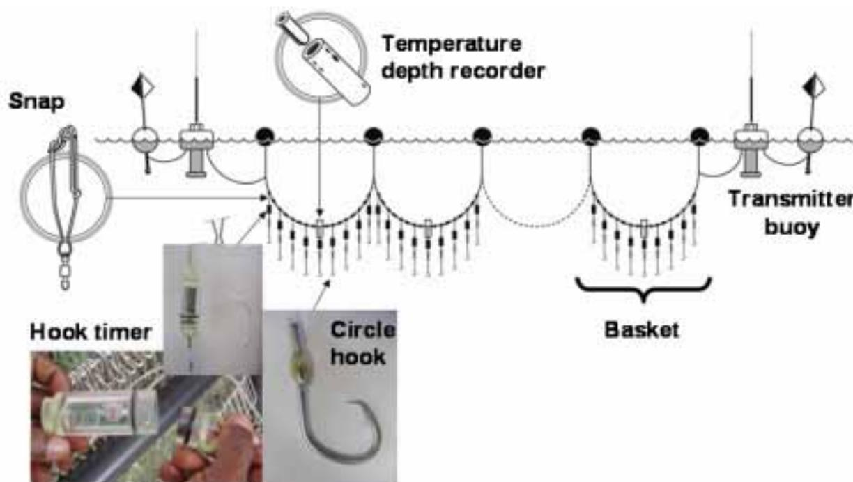
Figure 6 - The instrumented longline deployed during the SWIOFP ILL training cruise
