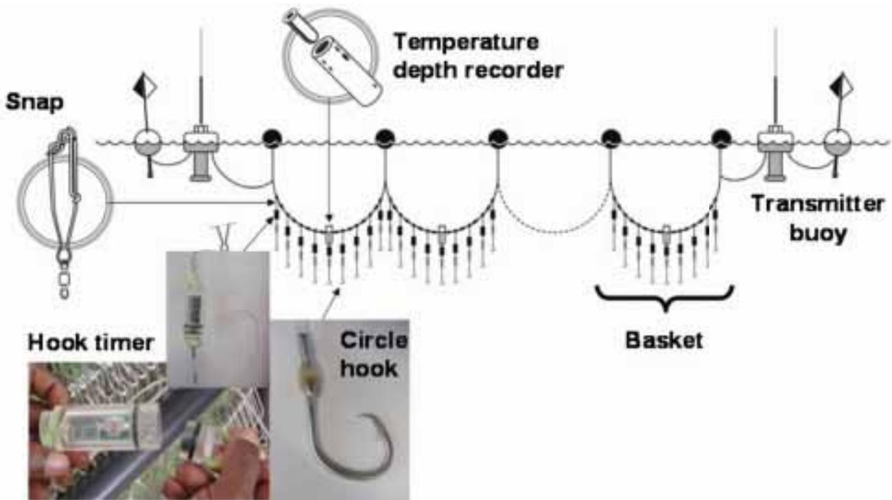
Figure 7 - The instrumented longline deployed during the SWOPAT2 cruise.
