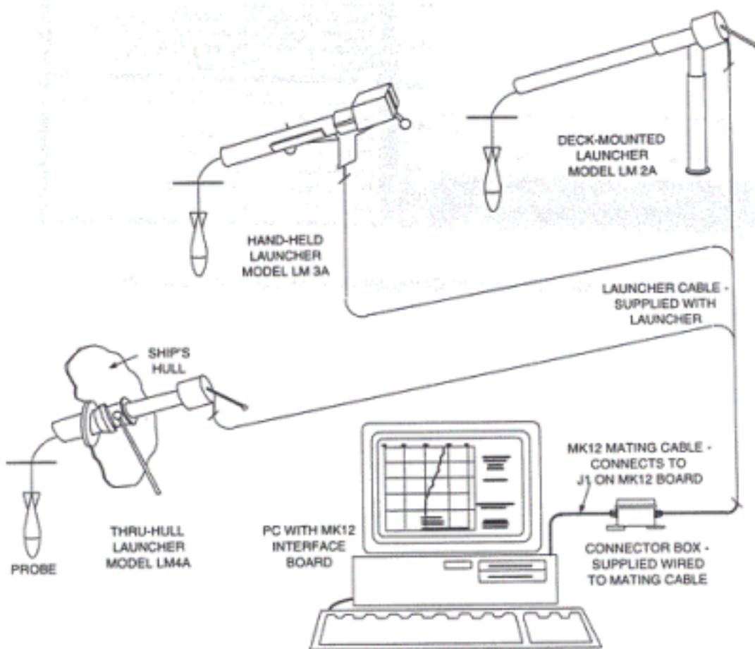
Figure 4 – Design of the Sippican's XBT system used to carry out temperature – depth profiles (Source : <http://www.sippican.com>).
