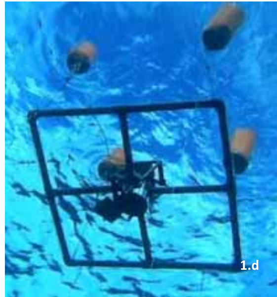
Fig. 1.c & 1.d: PVC frame equipped with a camcorder, 4 branchlines and 4 buoys
