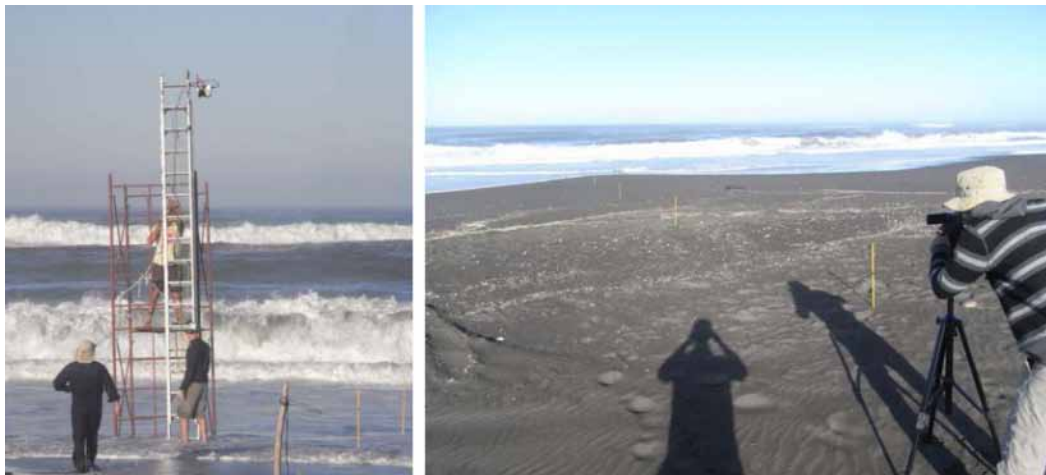
Figure 2, Swash hydro-morphodynamics measurements during the Mataquito dec 2013 experiment. a) LIDAR deployment on a scaffolding and b) optical video-poles setup.
