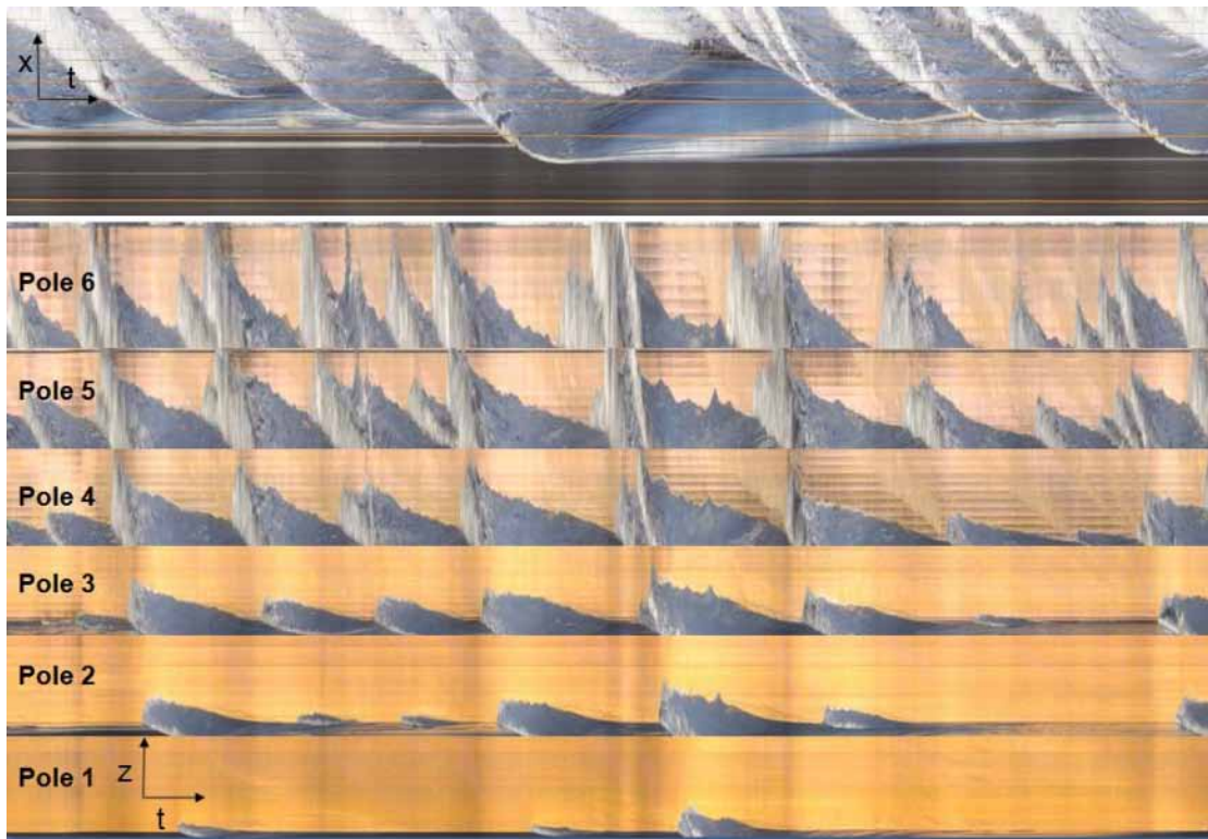
Figure 6, Video-pole technique illustration for Mataquito 2012 experiment. (up) cross-shore timestack showing the location of the 6 poles (yellow lines) within the swash zone. Lower panels show the vertical timestacks generated along the poles that allow monitoring the propagation of the waves and their deformation while they propagate to the shore. Vertical and temporal resolutions are \sim 0.001 m and 0.04 s, respectively.
