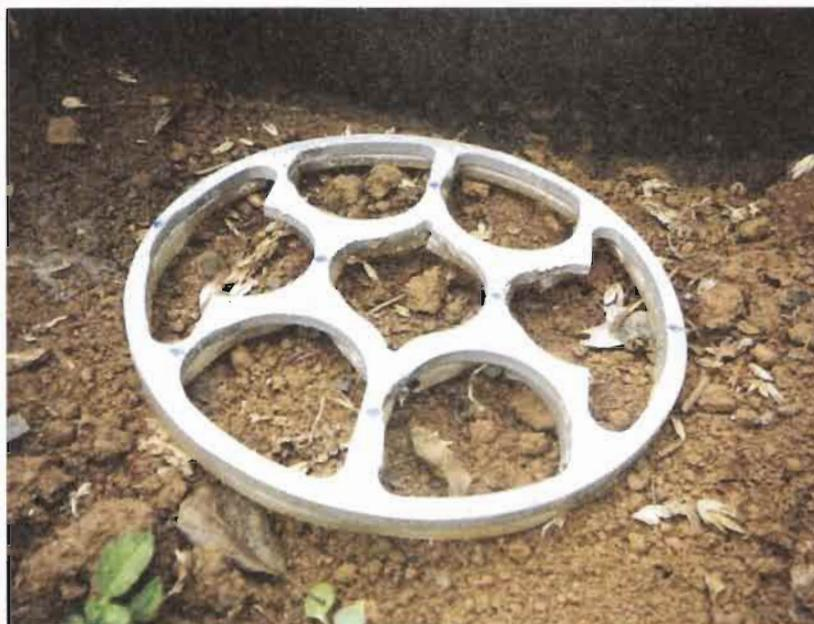
**Figure 2 –** Tube guide for the 7 infiltrating tubes.
