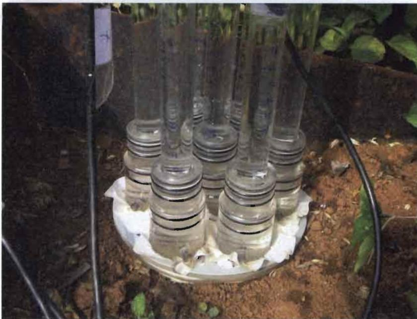
**Figure 4 –** The new infiltrrometer functioning
