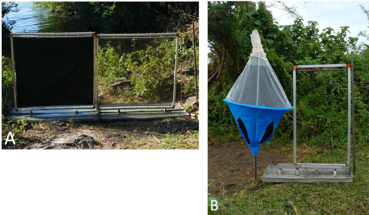
Figure 1. This shows the standard control devices against which new designs were compared. Each is flanked by an electric net to catch flies which circle the device but do not land. Electrified black target with flanking net (A) and a biconical trap with flanking net (B). doi:10.1371/journal.pntd.0001257.g001
