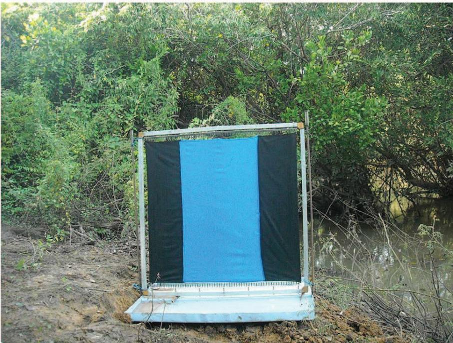
**Figure 2. The standard 1 m×1 m Black Blue Black e-target (treatment A) set up on a tray.**
