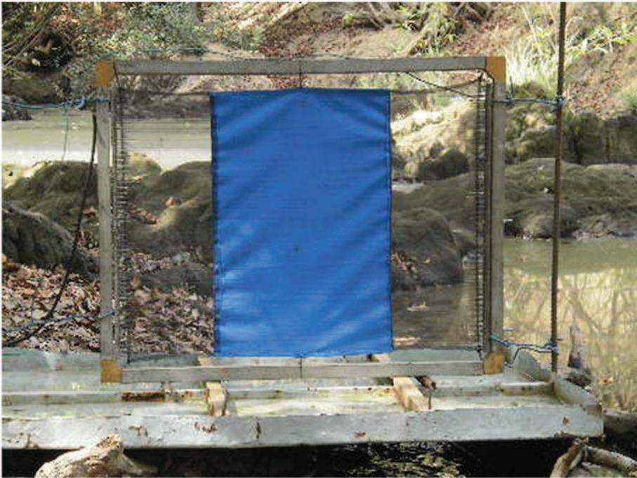
**Figure 1. Example of a target design used for comparison.** A 0.75 m wide×0.50 m high net-blue-net target (37.5 cm×50 cm blue surrounded by 2 pieces of net of 18.75 cm×50 cm each) inside an electric grid mounted on a fly collection tray.
