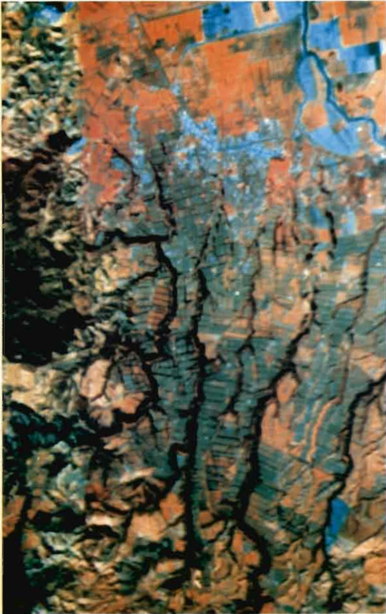
P14A : Simulated CIR enhanced colour composite subsce of Te Puke horticultural area from SPOT XS (443/426) winter scene taken on 5 August, 1986 at scale 1:100,000 compare with figs. 3 and 4. Colour tones: grey - kiwifruit; pink - pasture ; cyan large areas - fallow; mixed cyan and pink patterns - urban Te Puke; dark red - citrus; dark brown-red - native forest ; thin dark lines - evergreen shelter-belts. Note the dissection of the relatively flat broad inter-fluves by the narrow, deeply incised, bush-covered gorges. C CNES 86/dist SPOT IMAGE.
