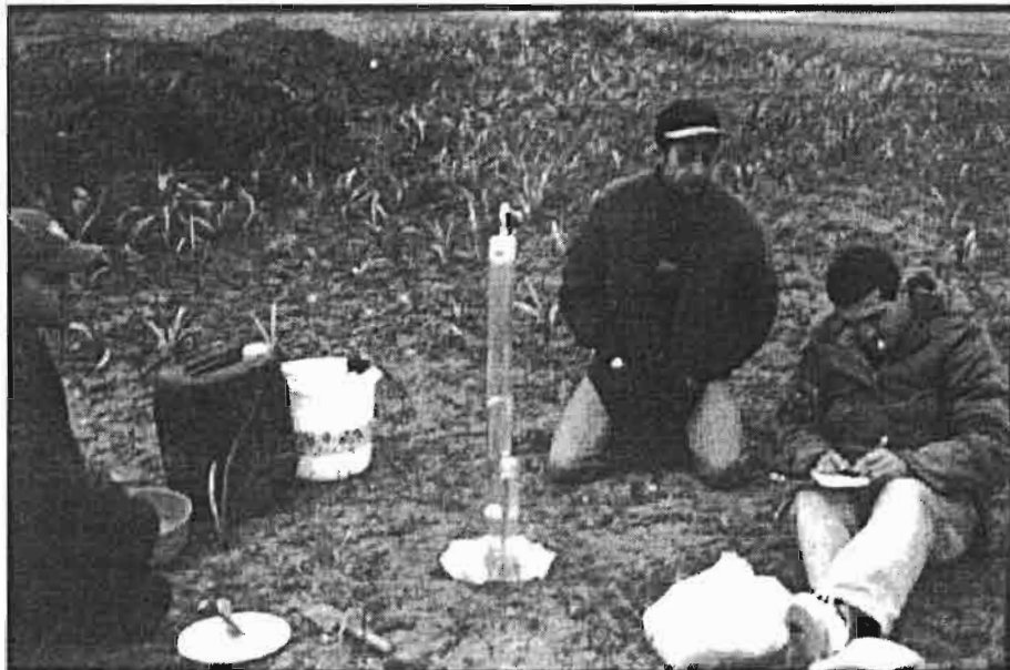
Measurement with the tension disk infiltrometer
