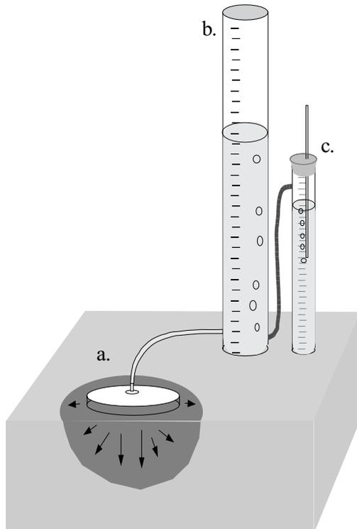
**Figure 1.** Schematic of a disk infiltrometer showing a. the actual disk on the soil surface allowing for 3D water flow, b. the water (or brine) reservoir and, c. the Mariotte device controlling the suction imposed at the soil surface
