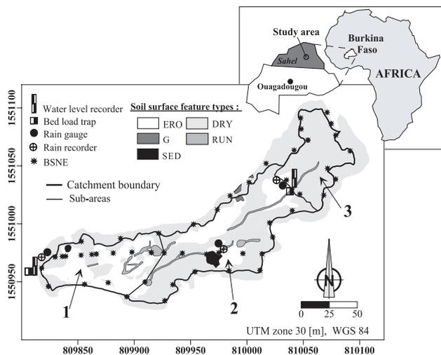
**Figure 1. The study area, map of soil surface features, experimental design and boundaries of the 2 catchments for which water erosion was calculated and of the 3 sub-areas for which wind budget was calculated**
