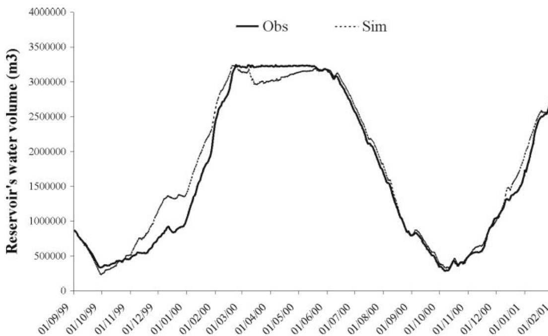
Figure 12. Observed and simulated Zongo reservoir water volume
