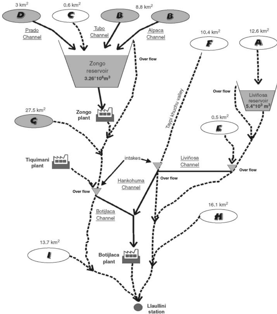
Figure 7. Schematic view of the hydroelectric system model built with Vensim<sup>®</sup>. The dashed lines represent the rivers and the solid lines represent the channels. The nine hydraulic catchments are integrated in the model. The grey-tinted catchments runoff is monitored and was not simulated with ISBA. Finally, all the water of the basin exits it at the Llaullini station
