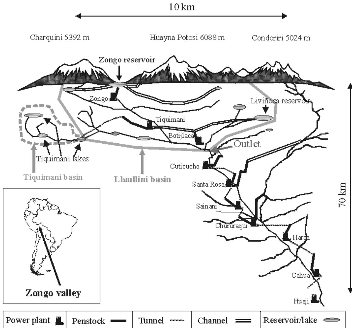
Figure 1. Schematic map of the Zongo valley hydroelectric system (reproduced with permission from COBEE, 1999)
