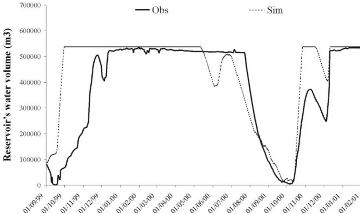
Figure 13. Observed and simulated Liviñosa reservoir water volume
