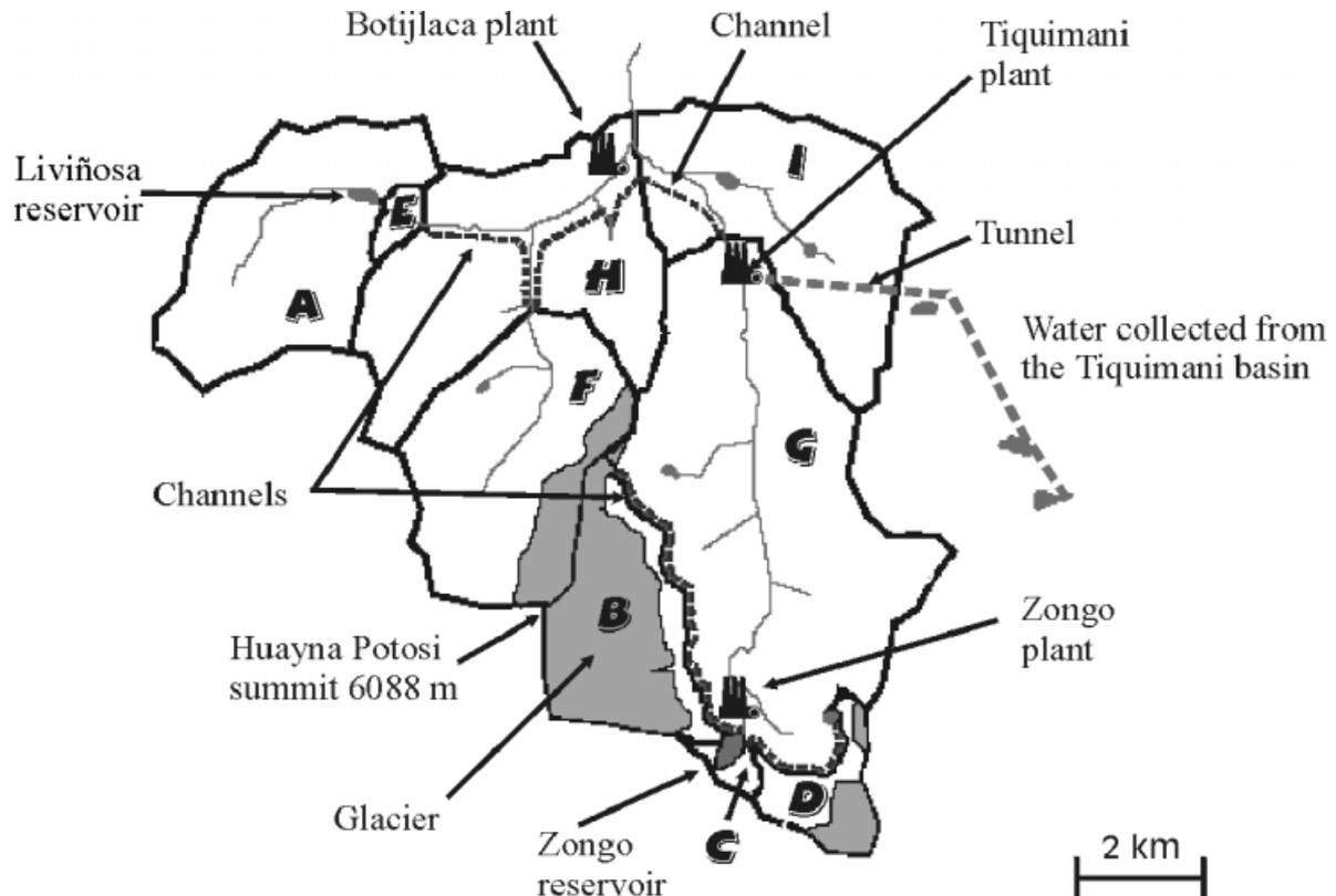
Figure 4. Limits of the nine hydraulic catchments identified by letters A to I, in the Llaullini basin. Channels, tunnels and reservoirs for the hydroelectric power plants are shown
