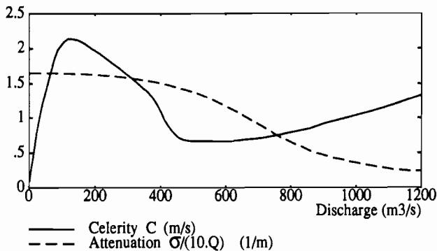
FIG. 4. Celerity and Attenuation Versus Discharge, for Erwood-Belmont Reach of River Wye [Attenuation is Plotted as Ratio  $\sigma/(10.Q)$ ]
