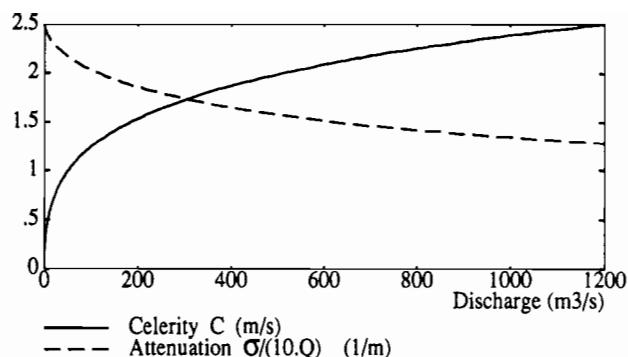
FIG. 1. Celerity and Attenuation versus Discharge for Hypothetical, Trapezoidal Channel [Attenuation Is Plotted as Ratio  $\sigma/(10.Q)$ ]
