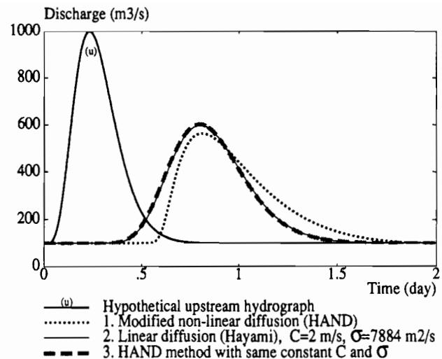
FIG. 3. Linear Versus Nonlinear Diffusion with Modified (HAND) Routing Method in Hypothetical, Trapezoidal Channel
