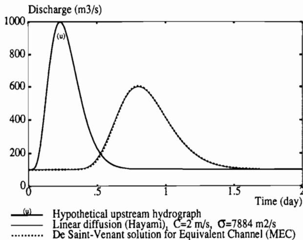
FIG. 7. Equivalent Channel (MEC) Method, Linear (Constant Coefficients) Case
