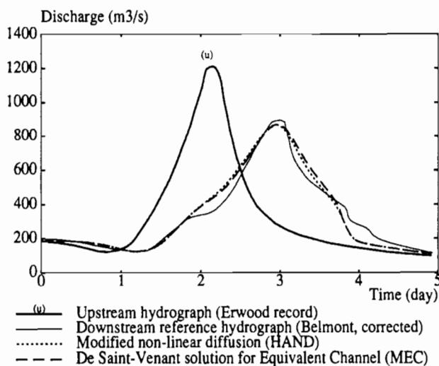
FIG. 8. Routing of December 1960 Flood by Equivalent Channel (MEC) Method, Erwood-Belmont Reach of River Wye
