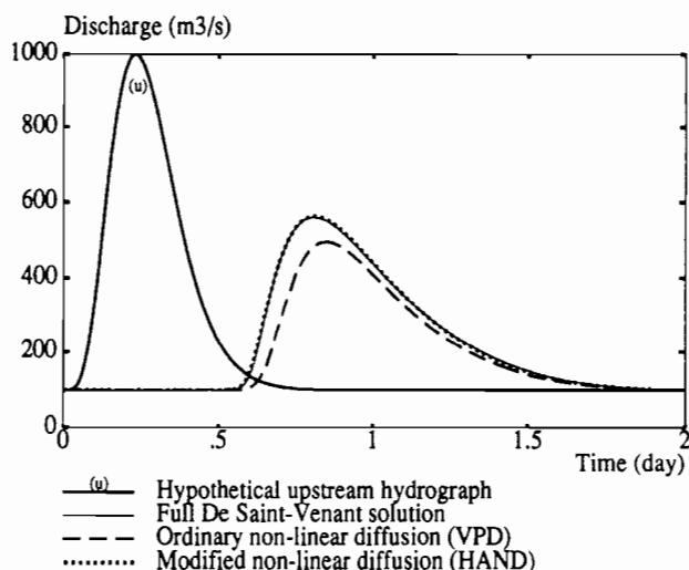
FIG. 2. "Ordinary" (VPD) versus Modified (HAND) Nonlinear Diffusion in Hypothetical, Trapezoidal Channel
