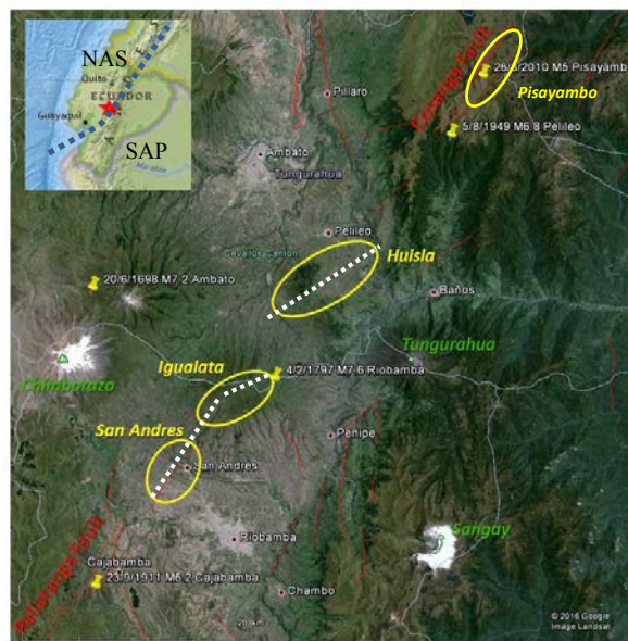
Fig. 1: Location of the study areas, between the known and mapped segments (Pallatanga Fault and Cosanga Fault) in red (fault traces from Alvarado, 2012). White dashed lines are fault traces investigated. Yellow pins locate the main historical earthquakes. In green, the major active or dormant volcanoes in the area. Insert: the blue dashed line depicts the shear zone that separates the North Andean Sliver (NAS) from the South-America Plate (SAP). Red star: study area.
