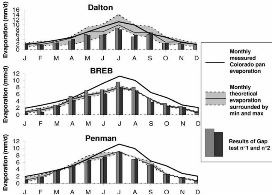
Fig. 3. Monthly evaporation determined with the BREB, Dalton and Penman methods (thin black line), bounded by the extreme values (grey area) and monthly Colorado pan measurements (thick black line) between 2003 and 2006; results of the two tests of robustness (Gap test n°1 and n°2).
