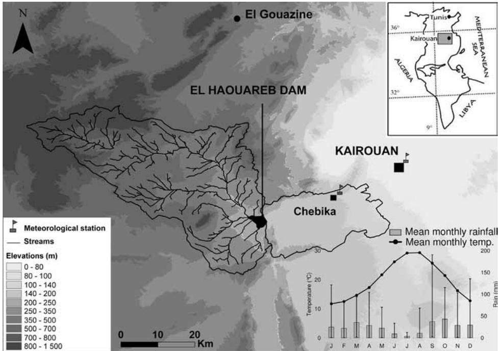
**Fig. 1.** Limits of the upstream and downstream Merguellil sub-catchments and location of the meteorological stations. The El Haouareb reservoir is the black shape. Chart of climatic characteristic of Kairouan: curve of mean monthly temperatures for 1957–2012 and bars of mean monthly rainfall for 1977–2009 with error bars showing extreme monthly rainfall.
