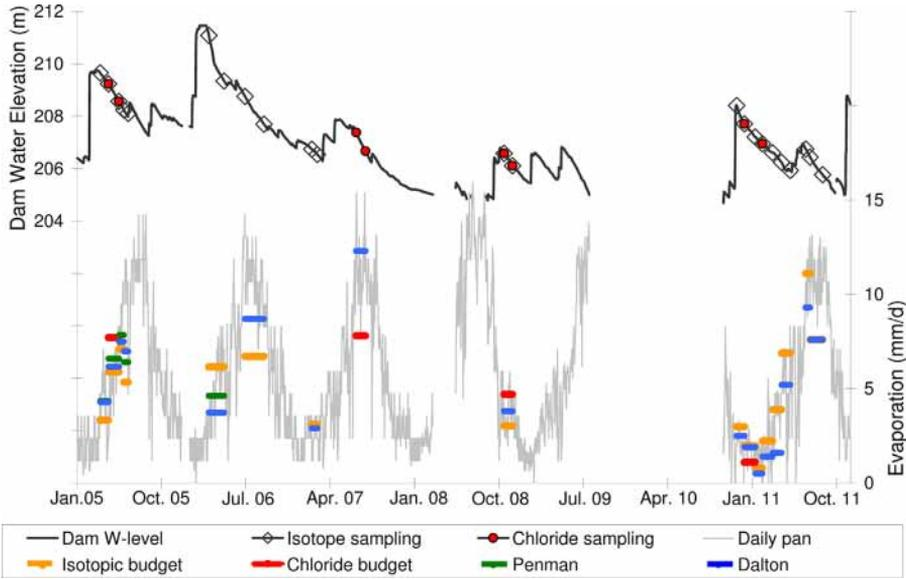
**Fig. 4.** Daily water level in the dam (black line) and measured evaporation at the Colorado pan (pale grey curve) from 2005 to 2011 with the dates of the isotope and chloride sampling (diamonds and red dots). Evaporation rates from the isotopic budget (orange symbols) chloride budget (red symbols) compared to evaporation rates calculated using the physical methods of Penman and Dalton (green and blue symbols).
