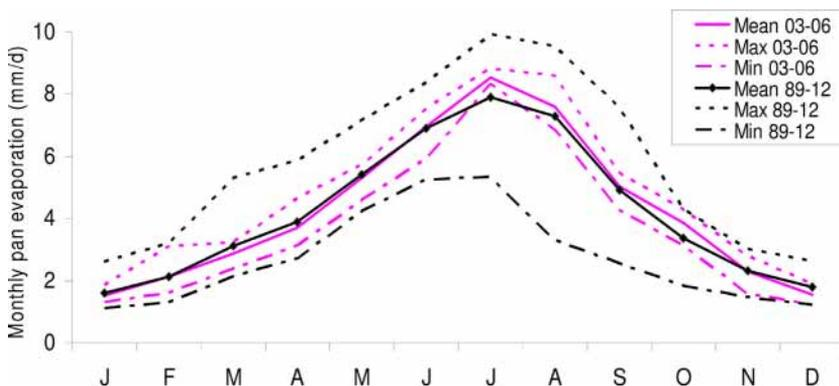
Fig. 2. Monthly means and extremes of evaporation measured in the El Haaoureb Colorado pan.
