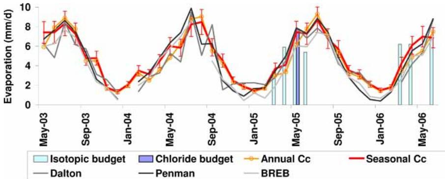
Fig. 7. Monthly evaporation determined using the Dalton, Penman and BREB physical approaches, occasional isotope and chloride budget, and the application of annual and seasonal  $C_c$  (with 15% error bars) for the period May 2003–June 2006 ( $\text{mm d}^{-1}$ ).
