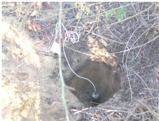
Fig. 2 Implementation of the measuring electrode in the hole
