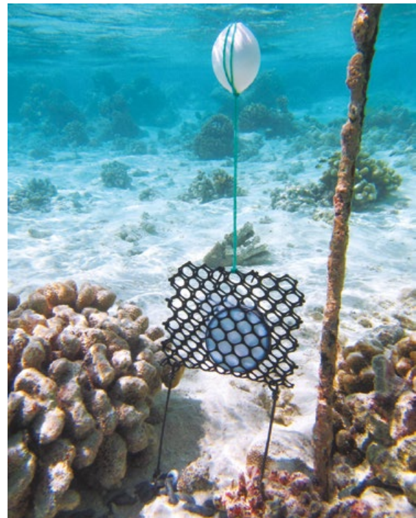
Figure 7. Deploying toxin-concentration devices (SPATT filters) in the wild. © ILM
