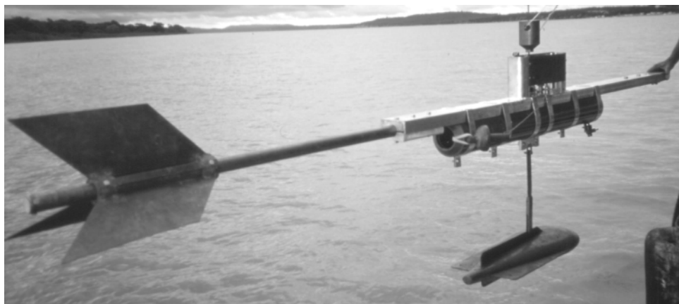
Fig. 2 The HiBAm sampler built from an oceanographic bottle, with a 12-litre nominal volume adapted to be used in big rivers.
