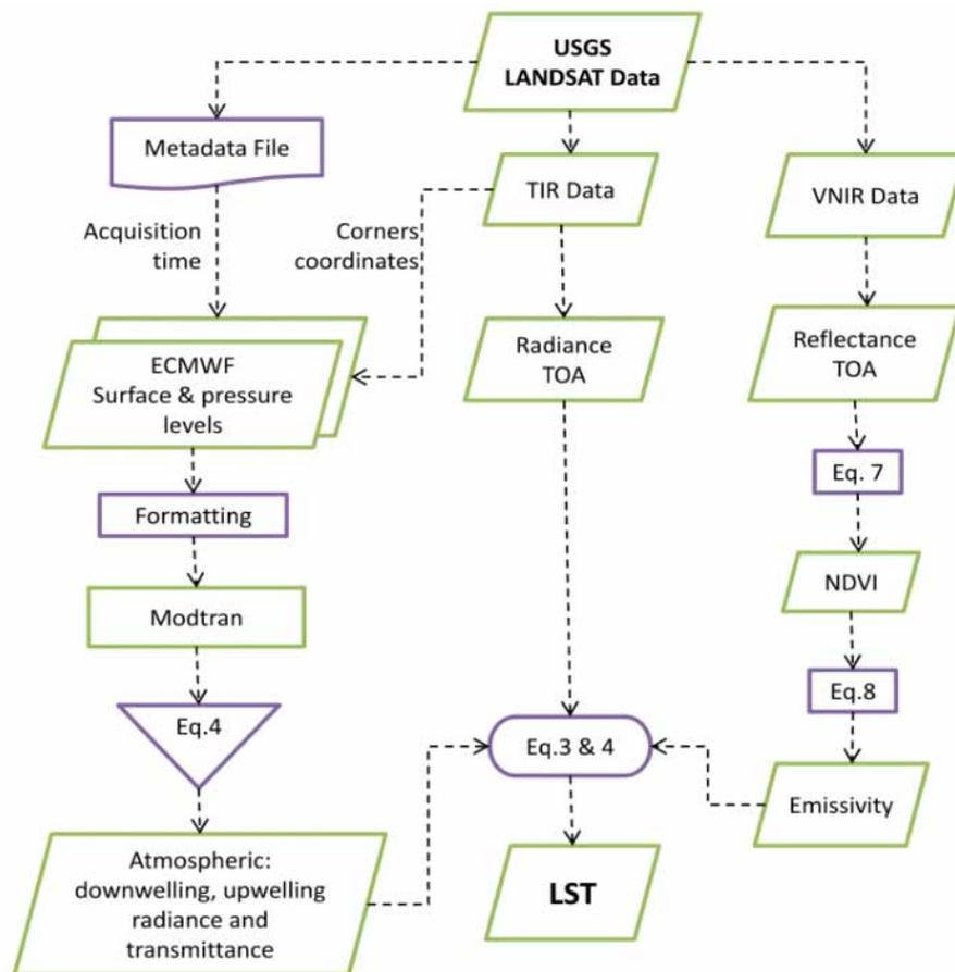
**Figure 2.** Flowchart of the LANDARTs algorithm to generate LST images at a resolution of 30 m.
