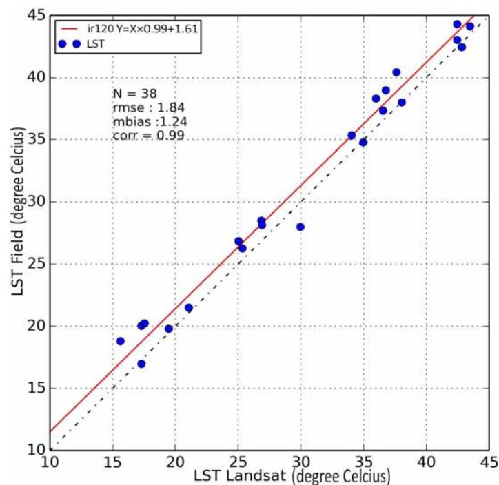
**Figure 3.** Comparison between Landsat LST and in situ temperatures (in degree Celsius) for the Tunisian site.
