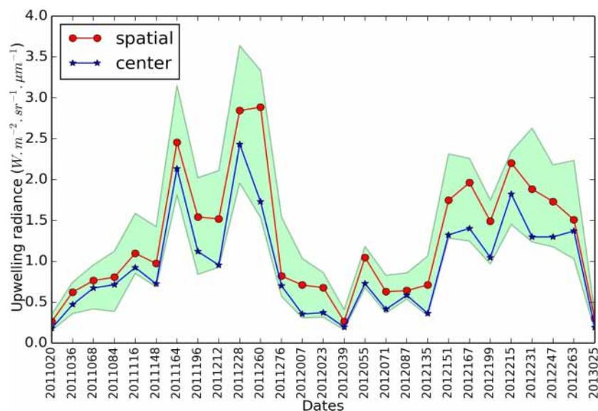
**Figure 13.** Multi-annual temporal evolution of the atmospheric upwelling radiance parameter ( $W \cdot m^{-2} \cdot sr^{-1} \cdot \mu m^{-1}$ ) observed for the set of French images (path/row 199/030). The blue line represents the center-scene upwelling radiance, and the red line is the upwelling radiance for the Aurade site extracted from the spatial parameter image at a resolution of 30 m. The green fill represents the amplitude (min/max) of the upwelling radiance for each Landsat scene.
