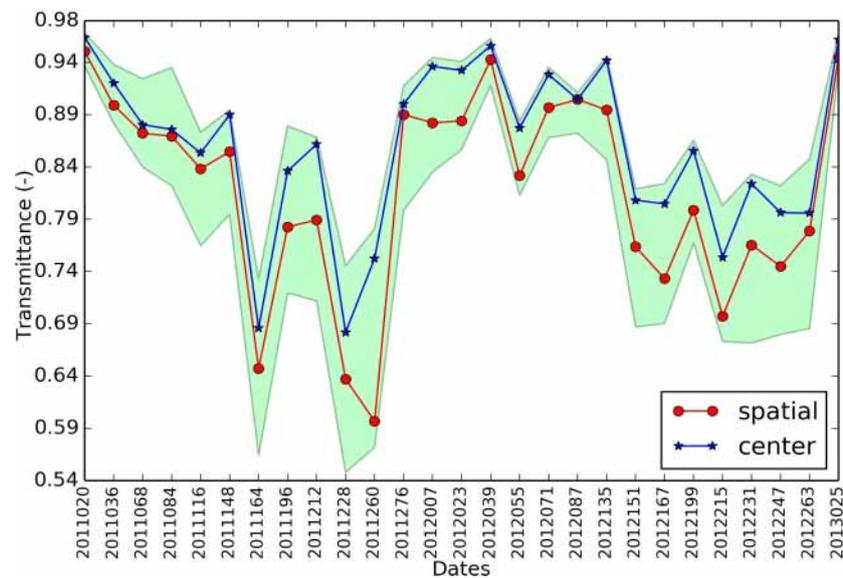
**Figure 12.** Multi-annual temporal evolution of the atmospheric transmittance parameter (unitless) observed for the set of French images (path/row 199/030). The blue line represents the center-scene transmittance, and the red line is the transmittance for the Aurade site extracted from the spatial parameter image at a resolution of 30 m. The green fill represents the amplitude (min/max) of the transmittance for each Landsat scene.
