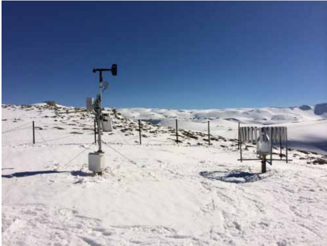
Figure 3. Automatic weather station at Mzar (MZA) (2296 m a.s.l.) where all sensors are located on the tower and the precipitation gauge is located to the right of the station. Image captured on 5 March 2015 (courtesy of the author).
