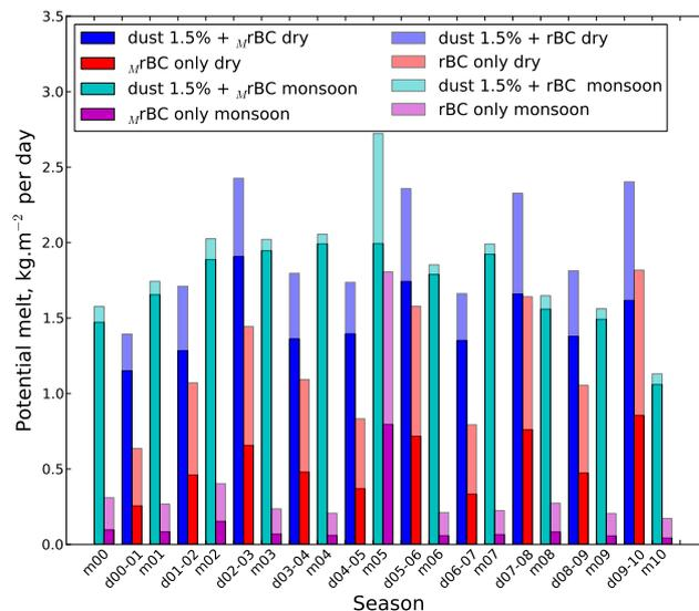
**Figure 8.** Potential melt per day due to the presence of impurities in the snowpack for each dry (for example d04–05 correspond to the dry season 2004–2005) and monsoon (for example m09 correspond to the monsoon 2009) season in the study. The hematite content used is 1.5 %. For each season, the first bar (blue or turquoise) corresponds to the presence of both dust and BC, the second (red or pink) to BC only.
