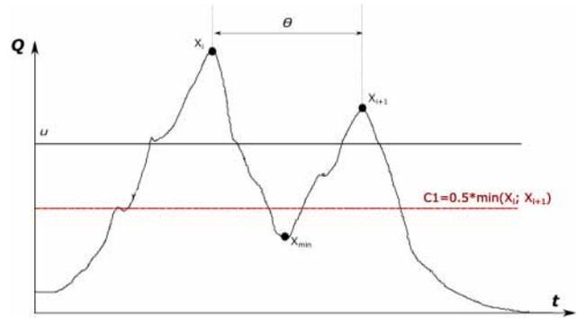
**Figure 4.** Extraction process of nPOT values.  $u$  is the threshold above which all peak are selected;  $\Theta$  is the time interval between two consecutive nPOT;  $X_{min}$  refers to the minimum daily discharge between two consecutive nPOT  $X_i$  and  $X_{i+1}$ ;  $C1$  is the minimum threshold between two consecutive nPOT.
