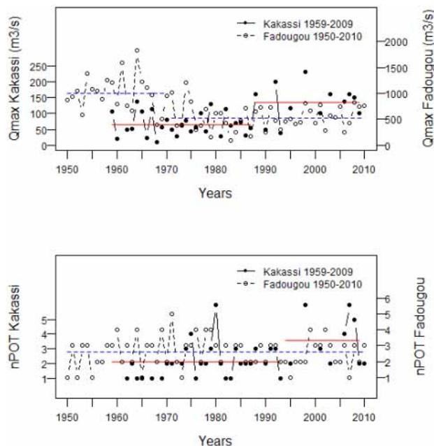
**Figure 6.**  $Q_{\max}$  and  $nPOT$  of long-term time series and segmentation according to the Pettitt break test. The dashed blue lines (solid red lines) represent the mean value of the flood index for each sub-period at Fadougou (Kakassi).
