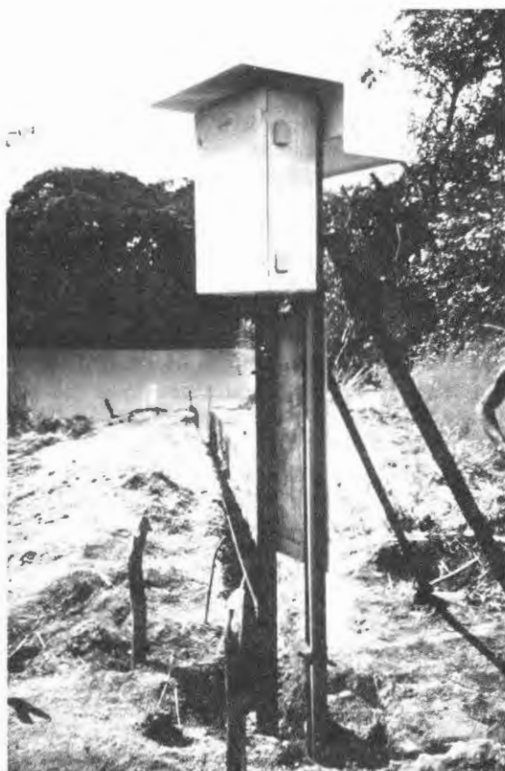
Fig. 2 The hydrological platform, with its solar panel, linked to the pressure sensor, on the Dion River, Diamaradou, Guinea (photograph by Michel Gautier, ORSTOM).
