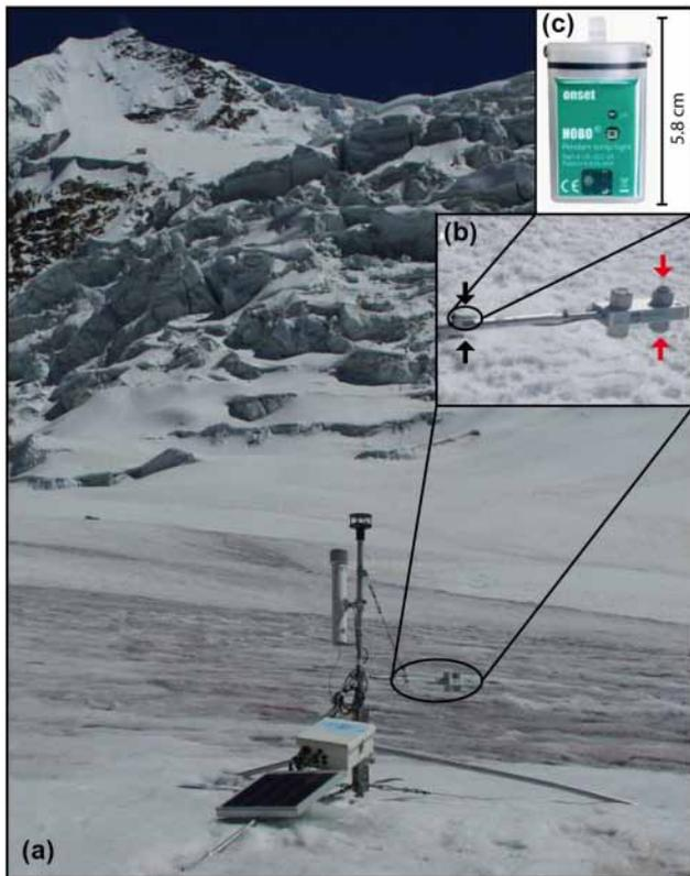
**Figure 1.** (a) Meteorological station on the Zongo Glacier; (b) CNR1 radiometer (Kipp & Zonen) installed at the SAMA meteorological station (the CM3 pyranometers are the two sensors on the right, red arrows) and the LCA comprised of two HOBO<sup>®</sup> Pendant Temperature/Light Data Loggers (black arrows); (c) zoomed-in view of a HOBO<sup>®</sup> Pendant Temperature/Light Data Logger (see Table 1 for detailed characteristics).
