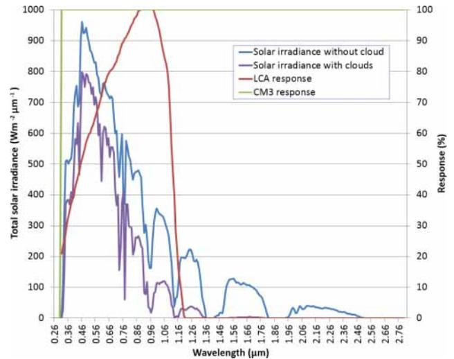
**Figure 2.** HOBO<sup>®</sup> Pendant Temperature/Light Data Logger and CM3 responses as a function of the wavelength and two examples of total solar irradiances for a clear sky (in blue) and for a cloudy sky (in purple) given by the DISORT model (Stamnes et al., 1988;  $\text{W m}^{-2} \mu\text{m}^{-1}$ ).
