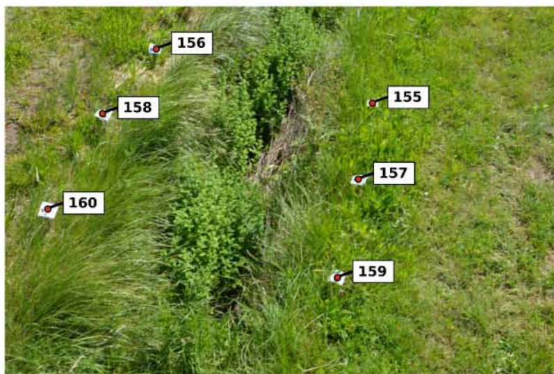
Figure 3. Illustration of automatic recognition of the targets on a picture using Photoscan Pro®. (a) original image; (b) image with recognized targets (boxes linked to a red dot).
