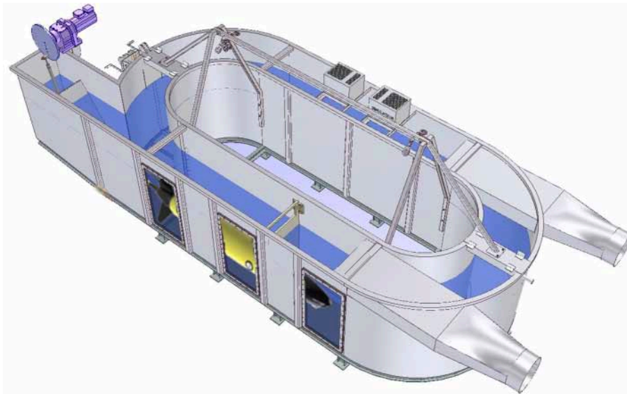
FIGURE 1 | Sketch of the “polludrome” at the Center of Documentation, Research and Experimentation on Accidental Water Pollution (CEDRE). The glider equipped with MiniFluo-1 and MiniFluo-2 was placed as illustrated here. Source of original image: G2B / CEDRE (modified with permission).
