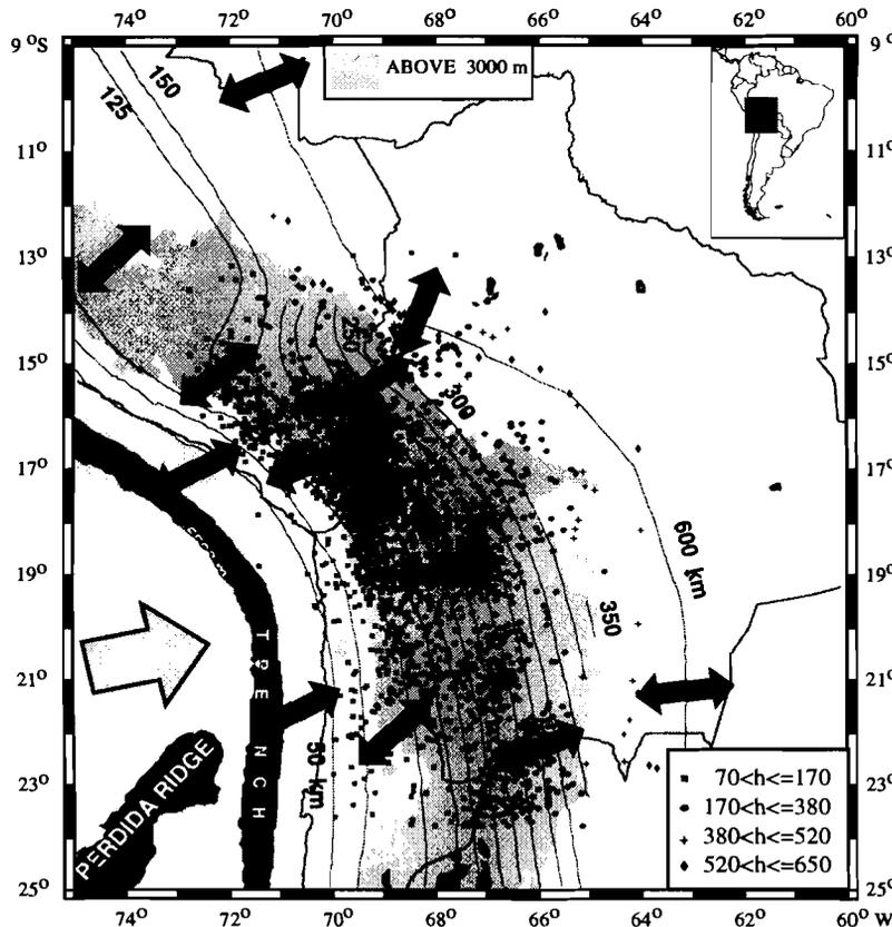
Fig. 3. Map showing the located intermediate and deep seismicity (from 70 to 640 km depth); depth contours of the Wadati-Benioff zone are from Cahill & Isacks (1992). Divergence arrows indicate principal tensional stress direction ( $\sigma_3$ ) obtained from the inversion of focal mechanism solutions.
