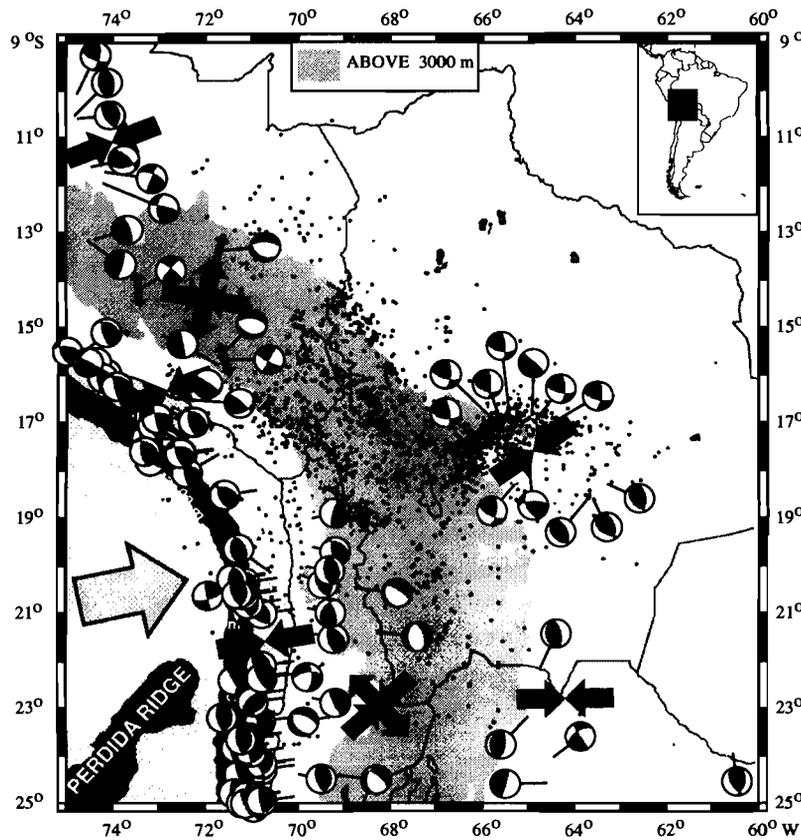
Fig. 2. Map showing the located shallow seismicity (less than 70 km depth). Balloons stand for lower-hemispheric projection of focal mechanism solutions. Convergence arrows stand for principal compressive horizontal stress direction ( $\sigma_1$ ); big divergence arrows for principal tensional horizontal stress direction ( $\sigma_3$ ) obtained from the inversion of focal mechanism solutions. The T-axes direction of tensional events for the High Andes is given by small divergence arrows.
