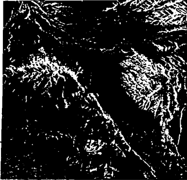
Fig. 4. Extraction of the Huaricangana fault line by mean of an upper thresholding of the SAR image.
