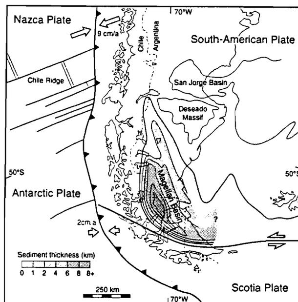
**Figure 1:** Map of southern South America showing tectonic setting with adjacent oceanic plates. Grey arrows indicate relative motions between plates. Sediment thicknesses in Magellan Basin are indicated in shades of grey (modified from Ramos, 1989).
