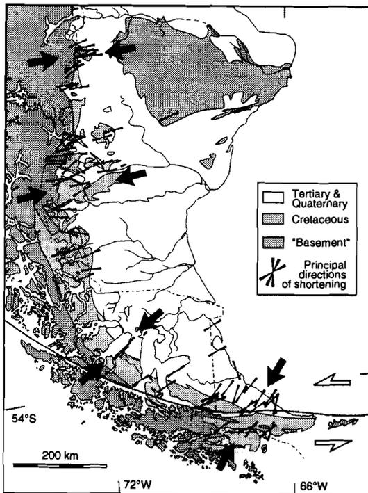
**Figure 2:** Schematic geological map with results of kinematic fault analyses at 74 localities. Small black arrows indicate calculated shortening directions. Large dark arrows summarize regional trends.
