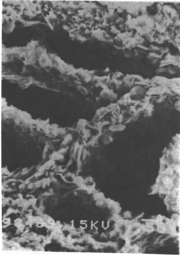
Photo X.1: Alveolar texture of Farinha Seca Bauxite (MEV-1200X).
