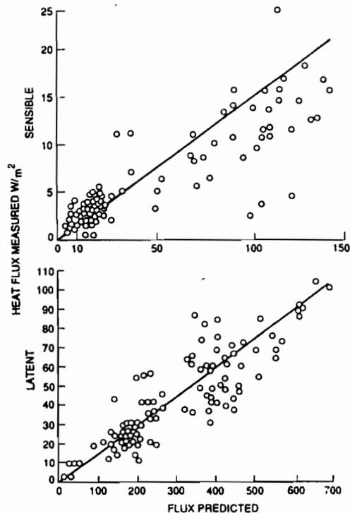
Fig 6 Comparison of field measurements of heat flux under free convection and values predicted by (6) (from Golitsyn and Grachov, 1988).
