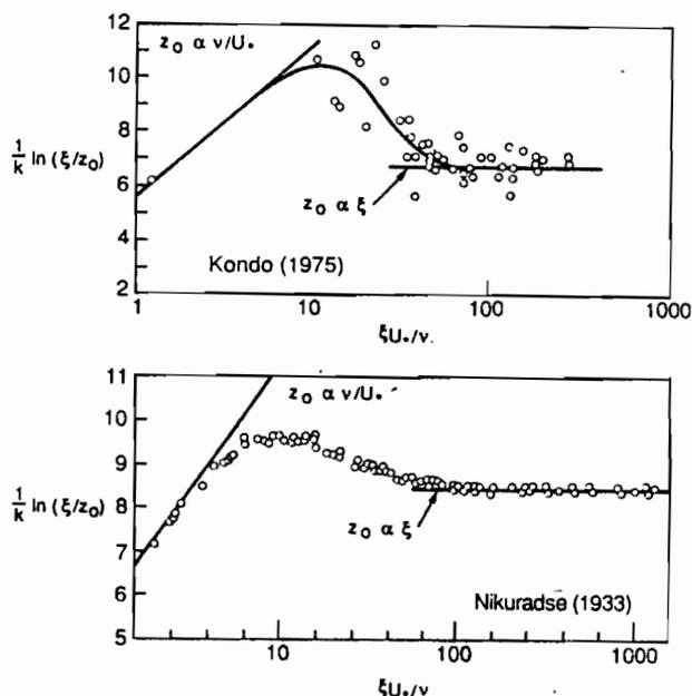
Fig.2 Variation of the roughness parameter in pipe flow (A) and at the sea-air interface (B), (from Liu, 1978).
