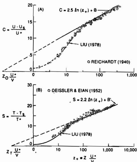
Fig.1 Laboratory measurements of the vertical profiles of (A) velocity and (B) temperature, (from Liu, 1978).
