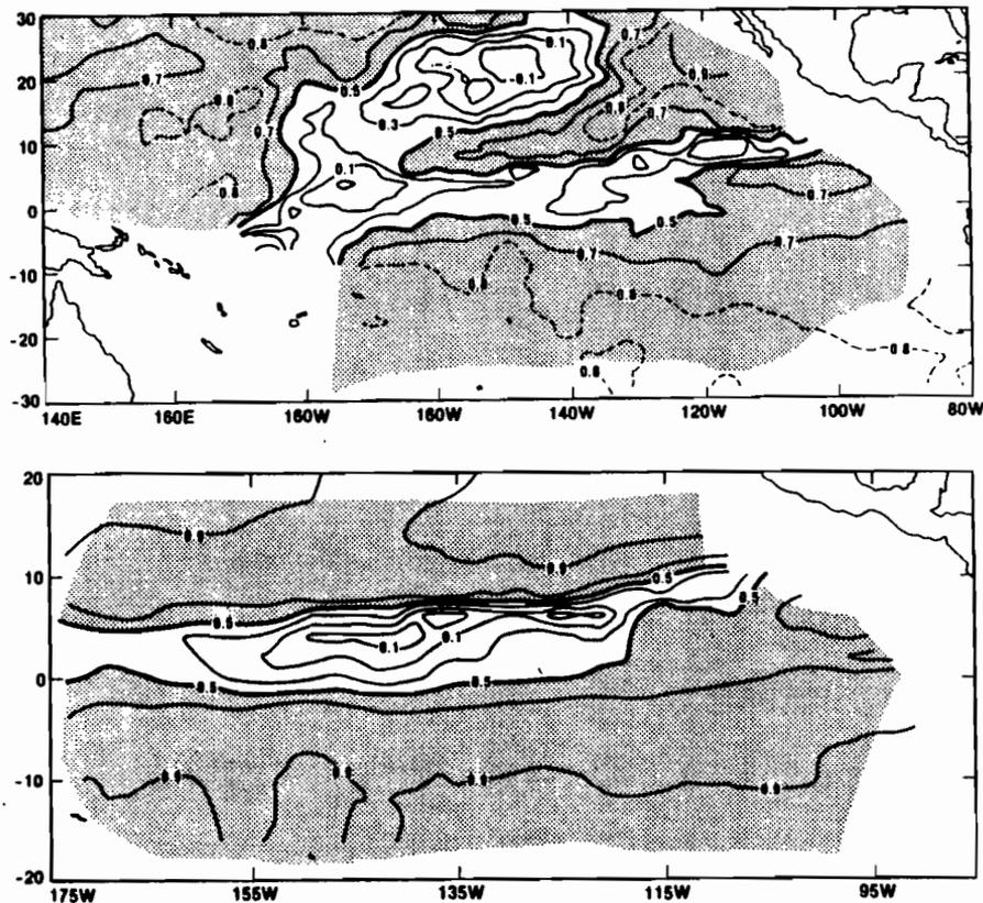
Fig. 8 Contemporary correlation coefficient between time rate of change of sea surface temperature and (A) latent heat flux (top), and (B) net heat flux (bottom). Solid isolines have 0.2 intervals.
