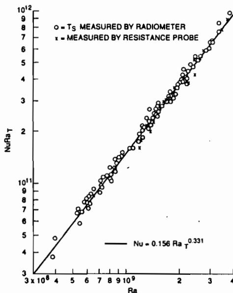
Fig 5 The relation between Nusselt ( $Nu$ ) and Raleigh Number for temperature ( $Ra_T$ ) for natural convection under a free surface (from Liu, 1974)
