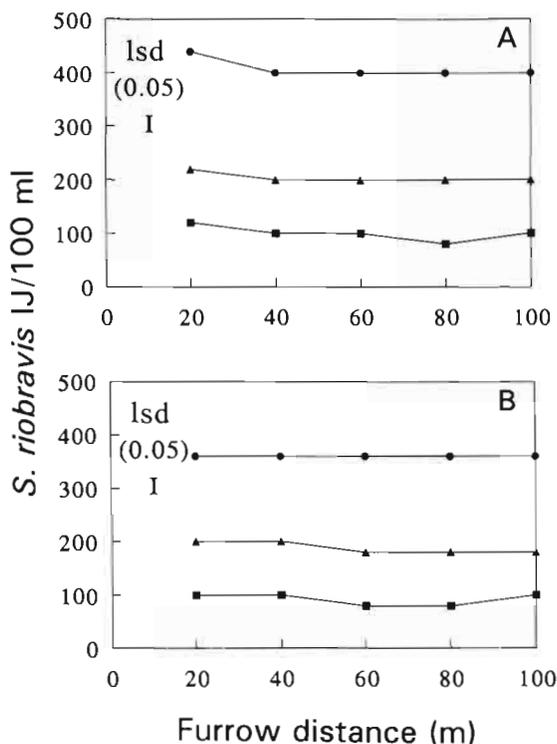
**Fig. 3.** Distribution of different concentrations of *Steinernema riobravris* applied via in-furrow irrigation along the furrow as expressed by the estimated numbers of infective juveniles transported by the irrigation water in corn field. A: During running water; B: Immediately after water had reached the furrow end (Numbers of nematodes are means of five samples/distance/concentration; ■ = 50 000, ▲ = 100 000, ● = 200 000 IJ/m<sup>2</sup>.)
