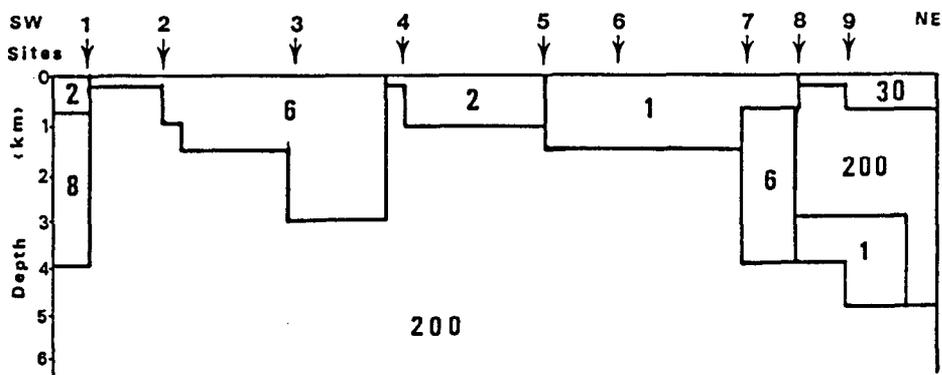
Figure 3. Two-dimensional resistivity model computed to model the MT traverse along the Bolivian Altiplano. Numbers indicate resistivities in ohm meters.
