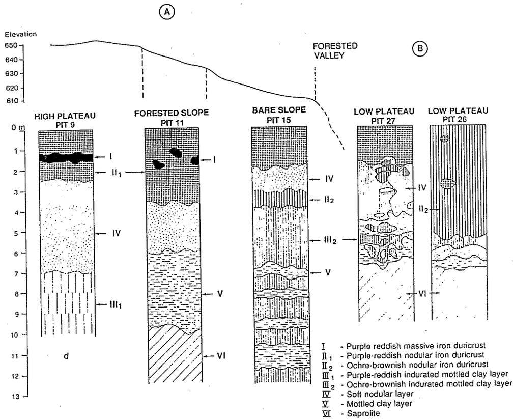
Figure. 2 - Sketch of weathering type-profile corresponding to (a) and (b) cross sections.
