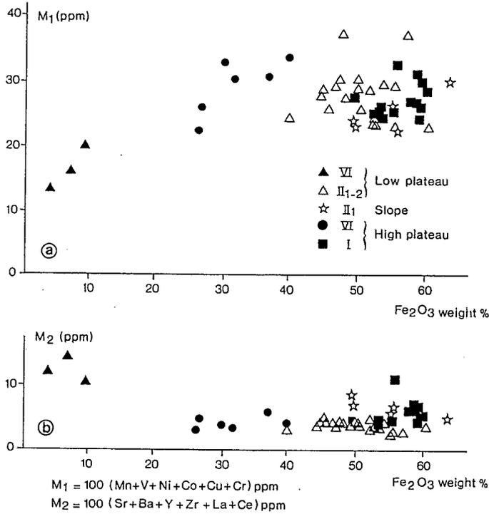
Figure. 3 - Trace element contents of saprolites compared to iron duricrusts (a - M<sub>1</sub> = 100 (Mn + V + Ni + Co + Cu + Cr) versus Fe<sub>2</sub>O<sub>3</sub>; b - M<sub>2</sub> = 100 (Sr + Ba + Y + Zr + La + Ce) versus Fe<sub>2</sub>O<sub>3</sub>).
