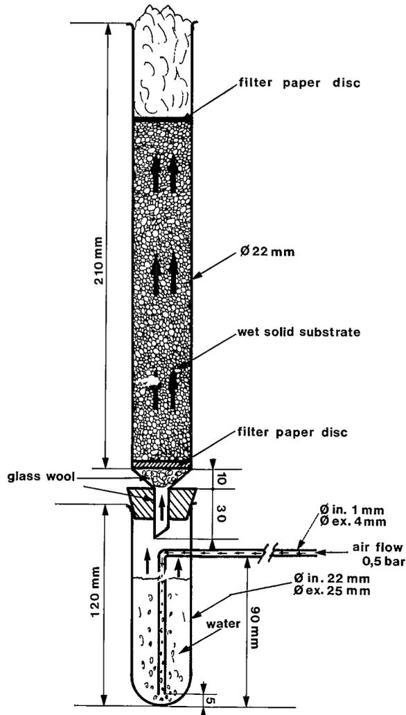
Fig. 1. Incubator device
