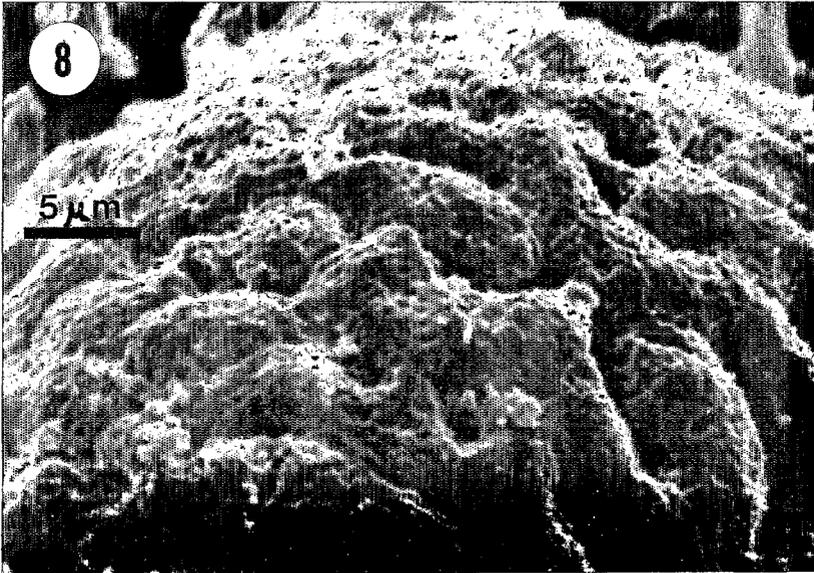
Fig. 7. Control sulfur granule treated with lead acetate
