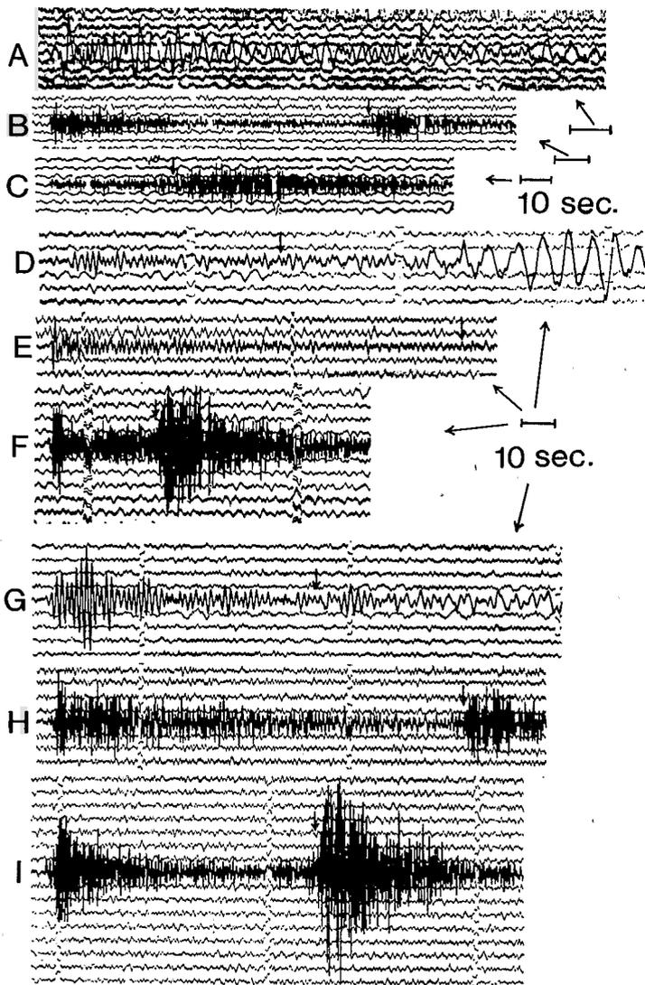
Fig. 2. Seismograms from LNR, PVC and NOU stations. A, B and C are examples from LNR; D, E and F are examples from PVC; G, H and I are examples from NOU. A, D, E and G are examples from shallow events of inefficient P- and S-transmission (dashed lines in Figs. 3, 4 and 5); B and H are examples from shallow events of efficient propagation (solid lines in Figs. 3 and 5); C, F and I are examples from mantle earthquakes of efficient P- and S-propagation.
