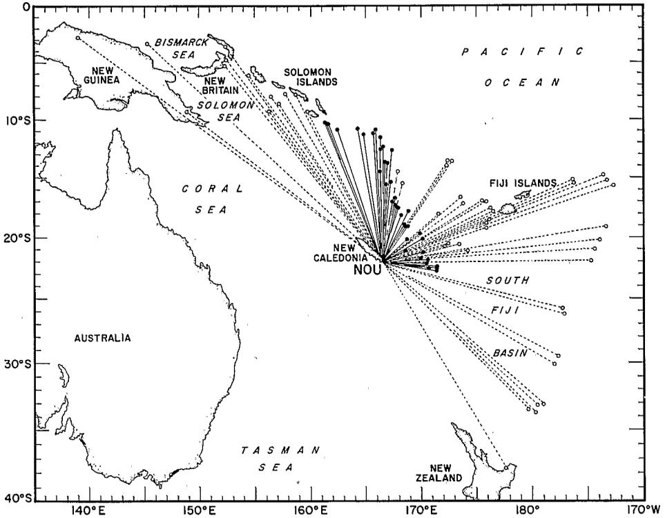
Fig. 3. Pattern of efficient and inefficient propagation of P- and S-waves from shallow earthquakes recorded at NOU (Noumea) in New Caledonia. Solid and open circles represent earthquake epicenters. Solid lines from solid circles to NOU represent efficient P- and S-transmission. Dashed lines from open circles to NOU represent inefficient P- and S-propagation.
