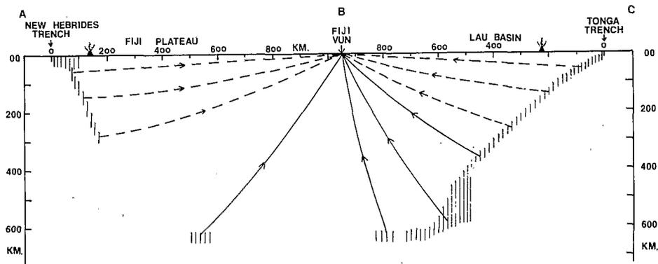
Fig. 6. Cross-section of Tonga and New Hebrides arcs (see Fig. 1 for the location of the section) showing location of seismic activity in the upper mantle (vertical lines) and representative ray paths to VUN in Fiji. Dashed rays represent paths where P- and S-waves are highly attenuated.
