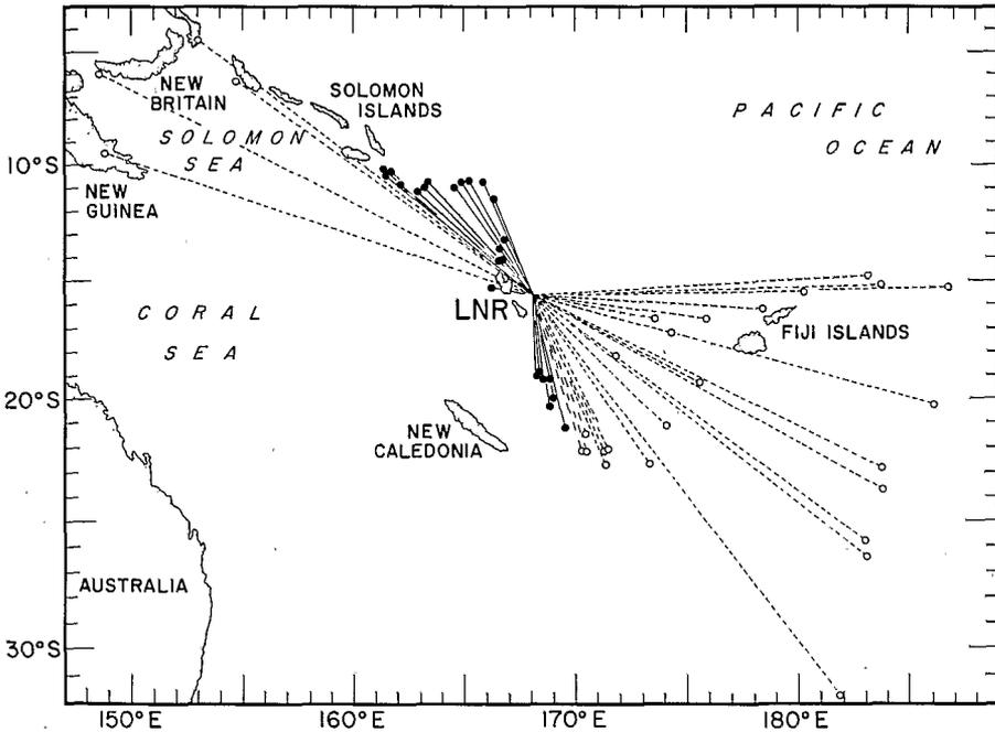
Fig. 5. Pattern of efficient and inefficient P- and S-propagation as found from the data of LNR (Lonorore) in New Hebrides. Symbols are the same as in Fig. 3.
