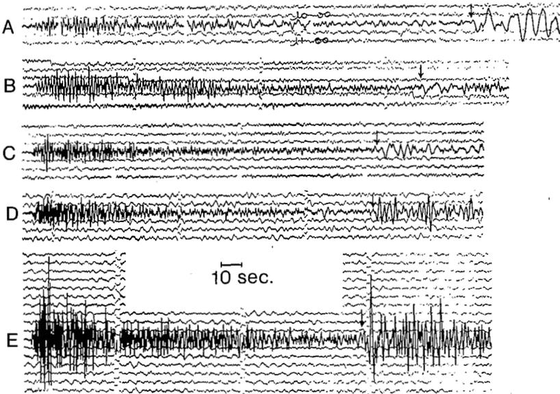
Fig. 7. Examples of seismograms recorded at NOU in New Caledonia from shallow, intermediate and deep earthquakes located along the Tonga-Kermadec seismic zone. The arrows on the records indicate the arrival times of S-waves.
