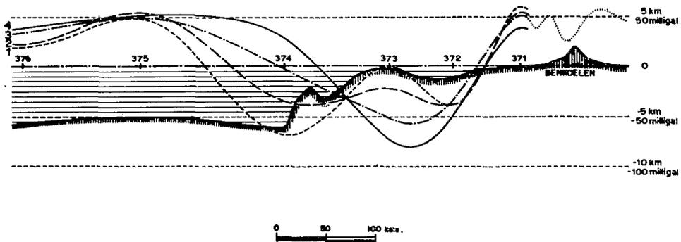
Fig. 3. Gravity profile of the Indian Ocean near Sumatra (over Benkoelen).
