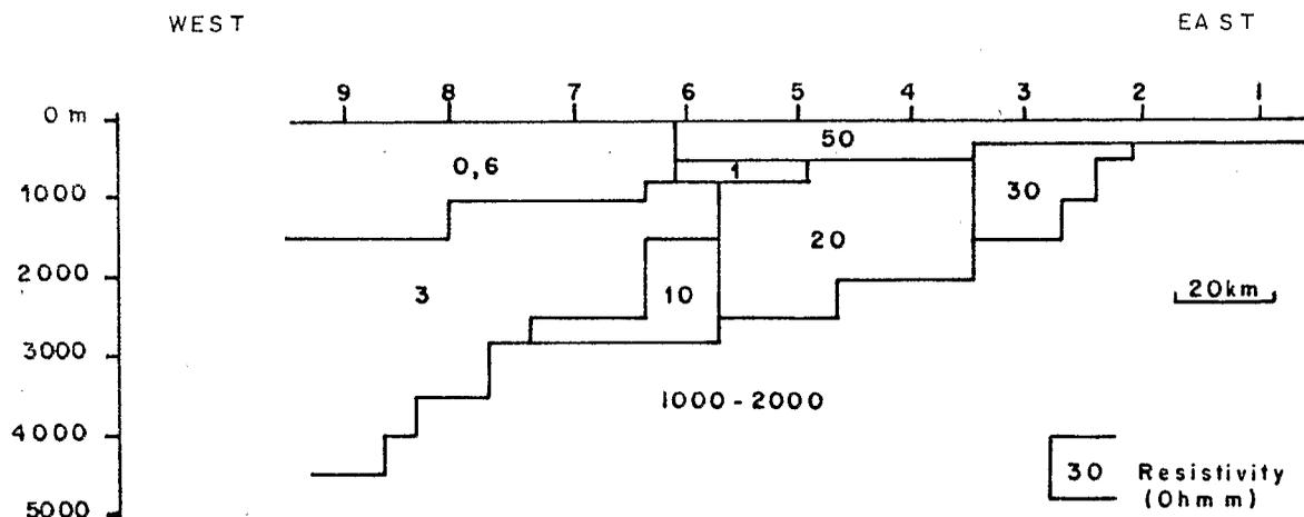
Fig. 2. Geoelectrical cross-section across the southern part of the S-M basin, constructed from MT soundings (after Ritz and Vassal, 1986).
