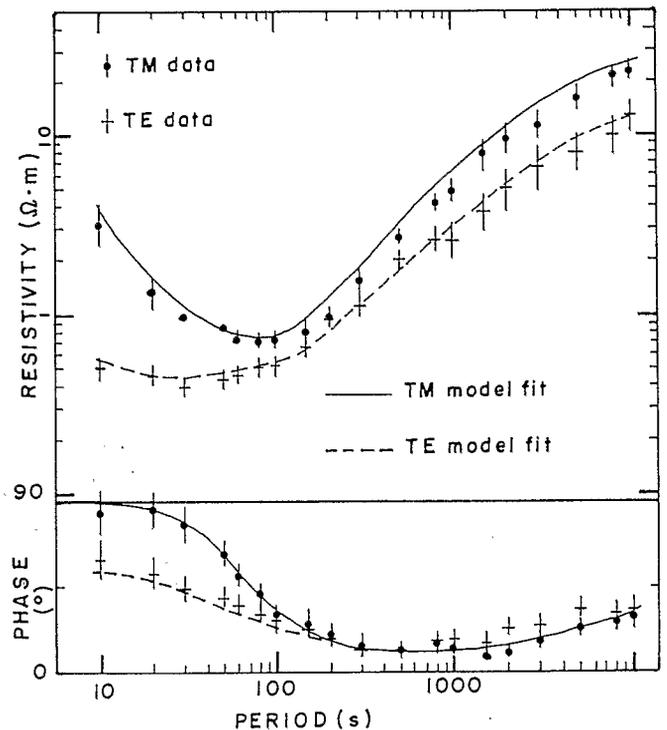
FIG. 2. MT sounding curves at site 8 on profile A-A' and fit of the two-dimensional model shown in Fig. 3 to the data.
