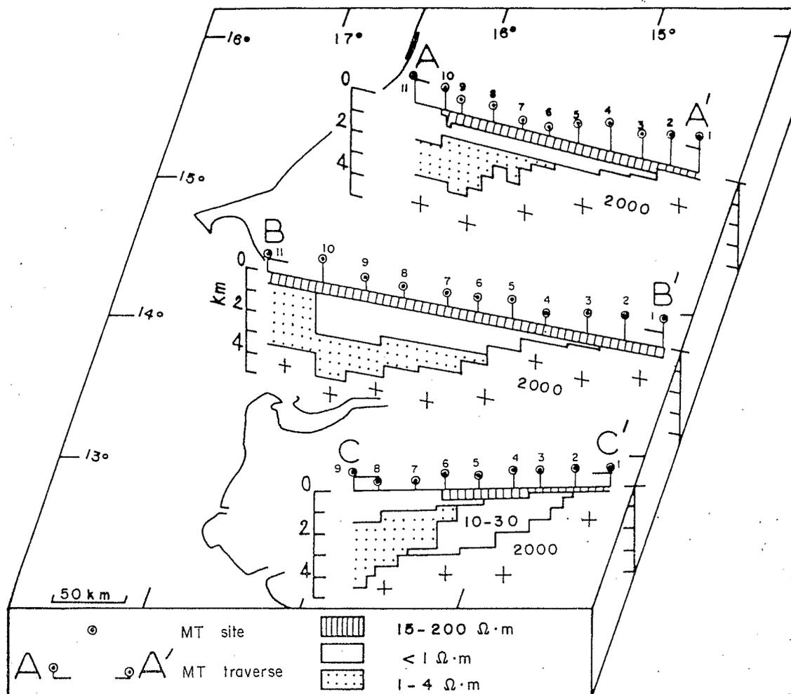
FIG. 3. Geoelectric cross sections across the Senegal-Mauritania basin compiled from the MT two-dimensional models. The numbers indicate the resistivities of the geoelectric units.
