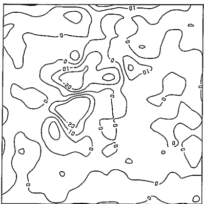
Fig. 7. Residual maps obtained by spline-laplacian method. The residual presents a high value in area of the pronounced slope.
