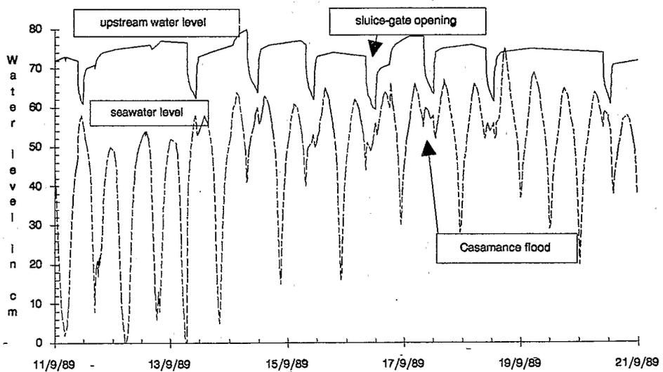
Figure 5 Upstream and downstream water levels at the anti-salt dam of Djilakou in September 1989.
