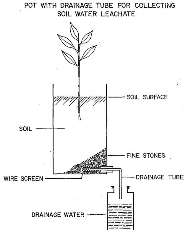
Fig. 1. Diagram of greenhouse pot system used for collecting aldicarb in soil leachates.
