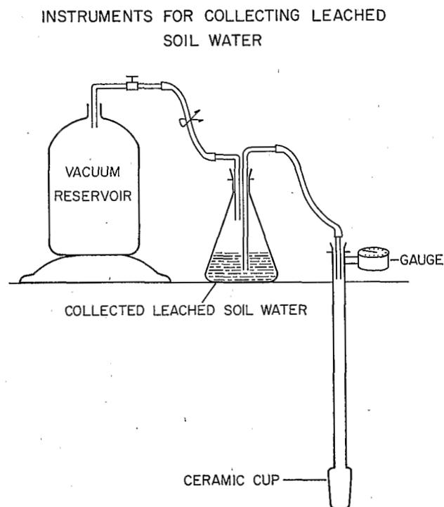
Fig. 2. Diagram of the field system used for collecting aldicarb in the subsurface soil water to a depth of 61 cm.
