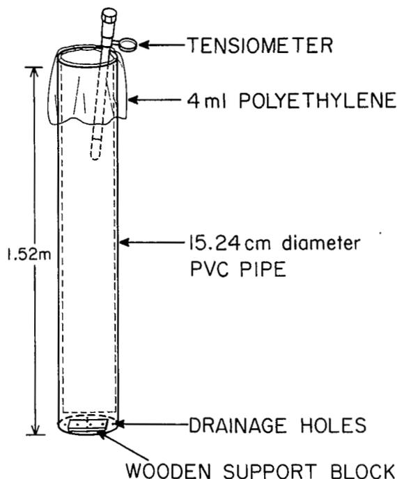
Fig. 1. P.V.C. tube with polyethylene liner and wooden basal support block.
