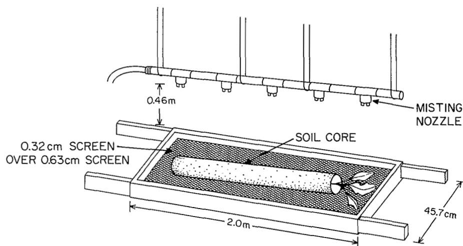
Fig. 2. Misting apparatus and supporting screens for removing soil from around plant root system.
