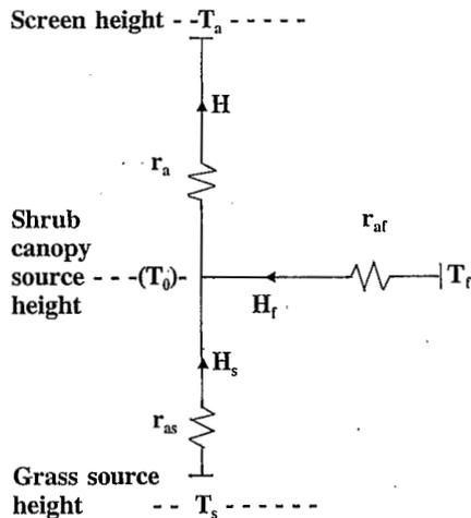
Fig. 1. Fluxes and potential-resistance network for a two-layer model of heat transfer from a Sahelian fallow savannah.  $T_a$  is air temperature at a reference height,  $T_f$  is shrub canopy temperature,  $T_s$  is substrate temperature and  $T_0$  is air temperature at canopy source height (aerodynamic surface temperature).
