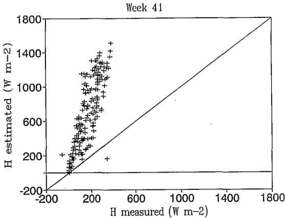
Fig. 3. For week 41 (DOY 279–285), comparison of sensible heat flux ( $H$ ) estimated using a one-layer approach with  $kB^{-1}=2$  vs.  $H$  measured by the energy balance–Bowen ratio system. The data are values integrated over 20 min from 08:00 to 17:00 UT. The line represents perfect agreement.
