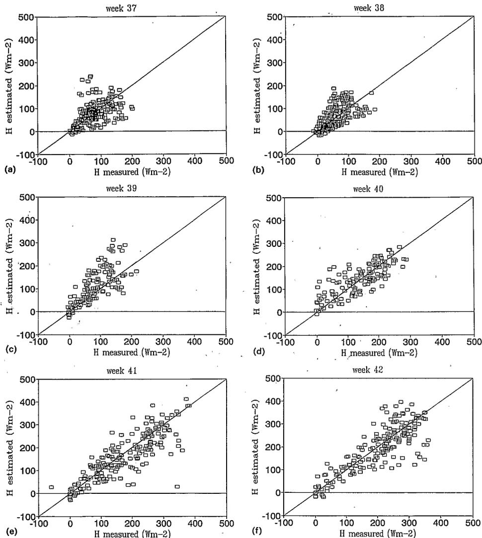
Fig. 4. Comparison of sensible heat flux ( $H$ ) estimated from Eq. (2) vs.  $H$  measured by the energy balance-Bowen ratio system for the 6 weeks of the experiment. The data are values integrated over 20 min from 08:00 to 17:00 UT. The line represents perfect agreement.
