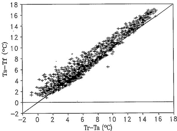
Fig. 5. The temperature difference between the substrate and the shrub canopy ( $T_s - T_f$ ) is plotted against the difference between surface radiometric temperature and air temperature ( $T_a - T_r$ ) for the whole set of data ( $n = 1019$ ). The data are diurnal values averaged over 20 min. The line represents perfect agreement.
