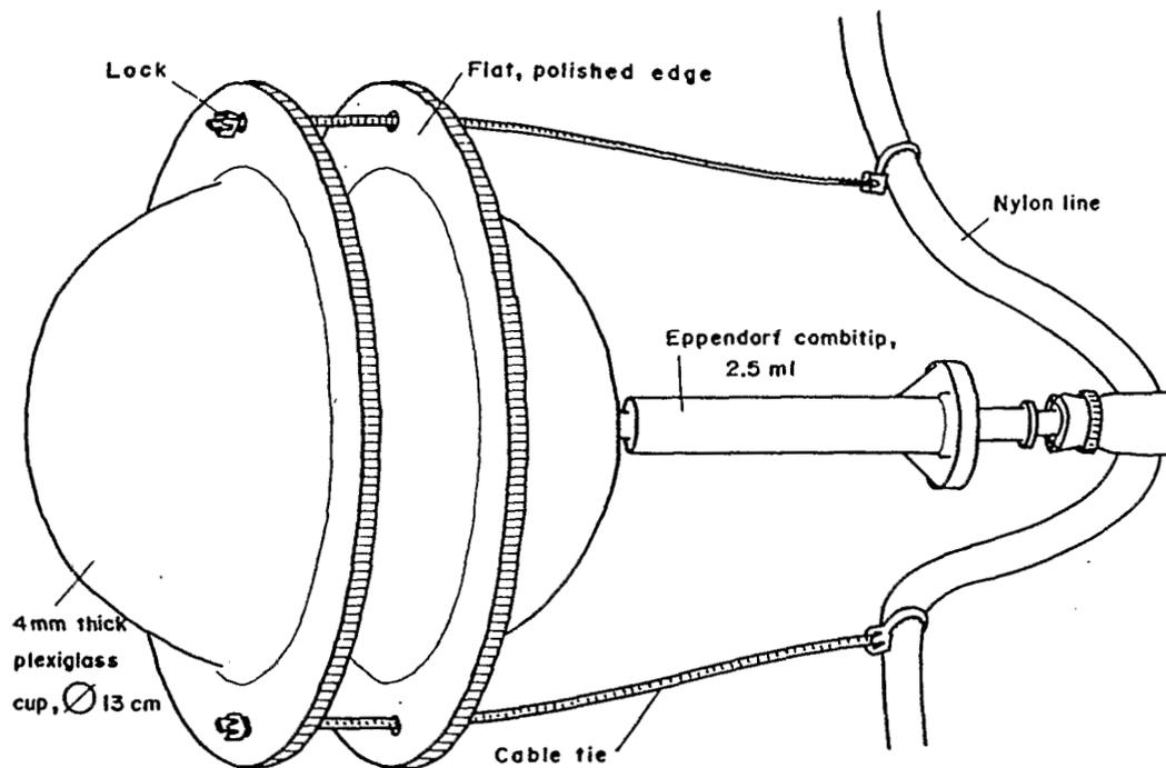
Fig. 2. Incubation cell. The plexiglass cups are formed with hot air blown over a mould at vacuum. The two locks (cut from other cable ties) are adjusted in such a way that the angle at apex B is about  $170^\circ$  when taut (see Fig. 1).
