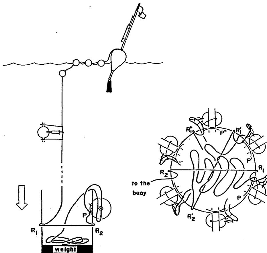
Fig. 3. Deployment of the LET GO setting at sea. Left: the line fastened to a buoy at the surface is delivered from the sinking bucket.  $R_1$  and  $R_2$  give way when the upper portion of the line becomes taut; the pin  $P$  is then pulled and the cell liberated. For sake of simplicity, only one cell is presented (the system has 12 cells). Right: top view of the bucket showing the fixation of the first row of cells through the wall of the bucket.
