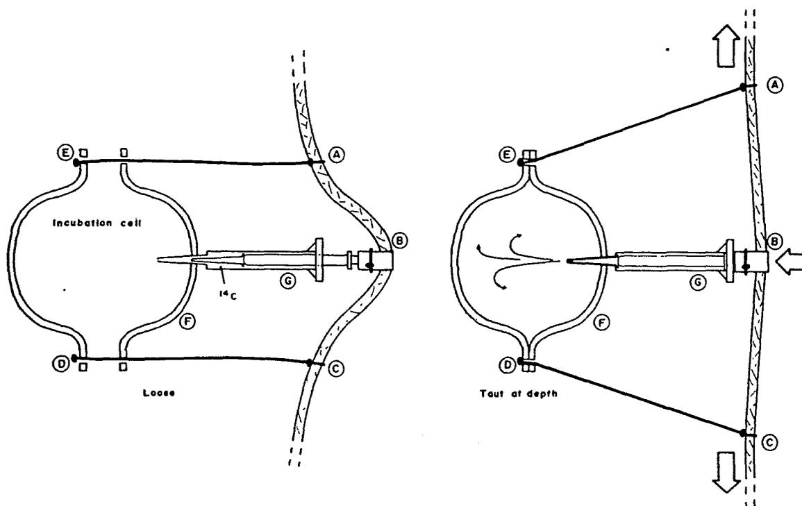
Fig. 1. Configuration of the LET GO incubation cells. Left: incubation cell prior to deployment. Right: when the line (ABC) gets taut, the pentagon ABCDE is deformed; the apex B pushes the cup F towards the opposite side DE, and operates the syringe G.
