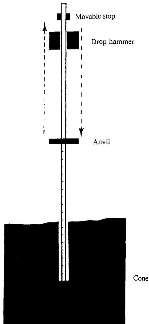
Figure 1. Diagram of a hammering penetrometer.
