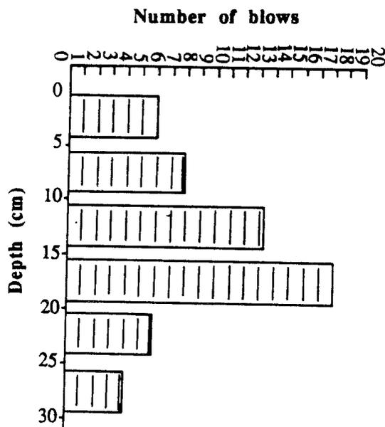
Figure 2. Example of a penetrometric profile established on site. Each bar represents a blow.
